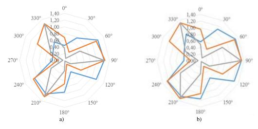
Fig. 4. The emf, Primary placed in delta, probe coil in vertical position: a) 20 V; b) 30 V.
