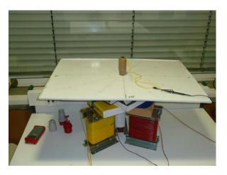
Fig. 2. Coils, platform and probe coil to conduct the tests.
