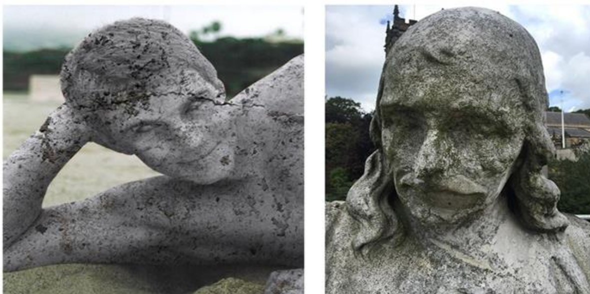
Figure 1. 16: Effects of cracking and sugaring on stone (Adapted from: www.tutorgrafico.com , www.hirst-conservation.com ).
