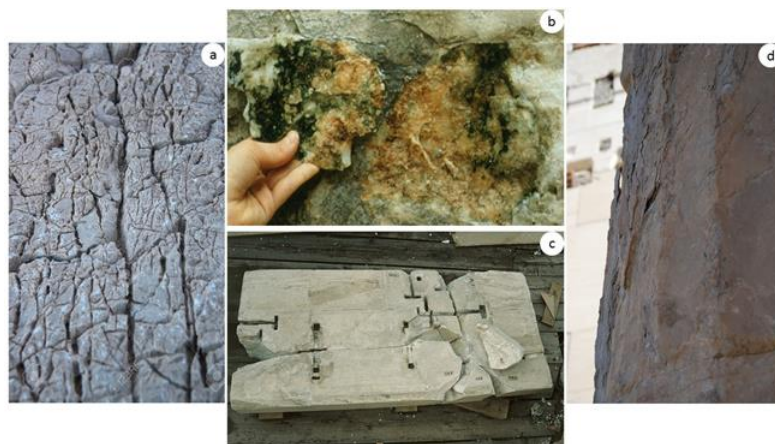
Figure 1.18: Effects of salting a) dislocation, b) breakage and c) flaking (Adapted from:
