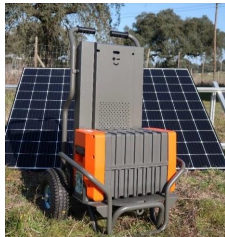
Figure 1: 2.0 kW/ 2.3 kWh second-life lithium-ion battery developed by betteries AMPS GmbH and installed in a pilot test as a result of the established cooperation between the University of Évora and betteries AMPS GmbH .
