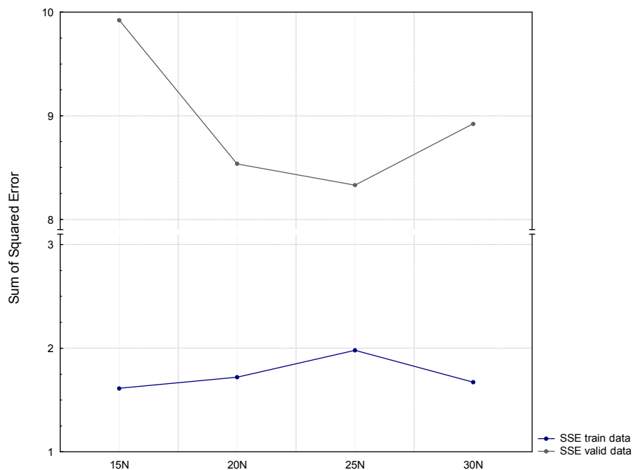
Figure 20 – Sum of squared errors of the training and validation data by the different ENN architectures tested for Myotis species classification
