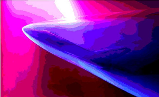
NASA: Visible shocks at the nose in the windtunnel test
