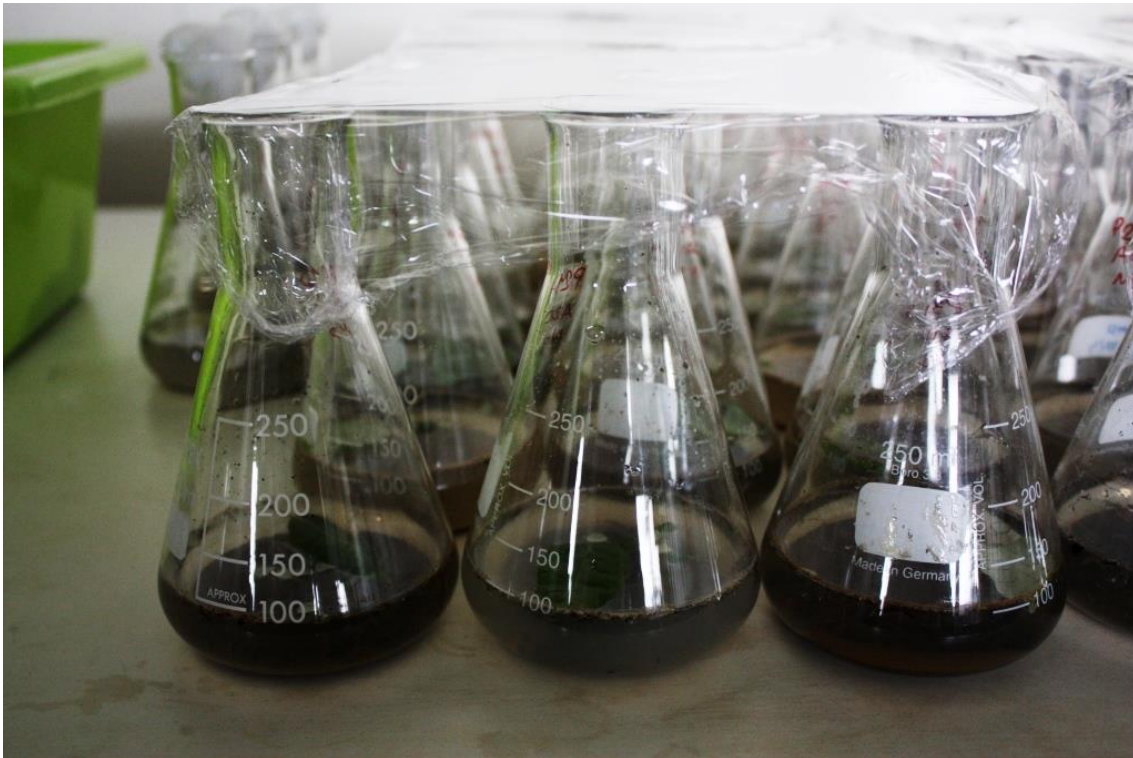
Figure 4.4: Baiting method: 25 g of soil submerged in 100 ml of water, with floating cork oak discs to bait Phytophthora cinnamomi zoospores.
