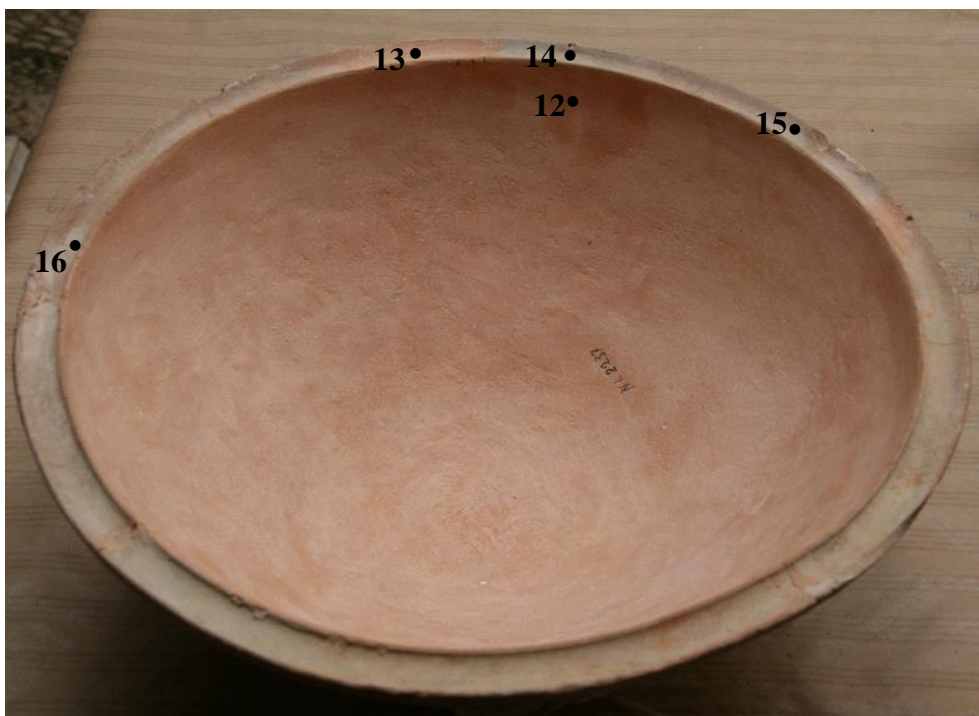
Fig. 5: XRF inside lid points from different colored areas in vase A. the colors are as following: white points (16); orange point (12,13); grey points (14,15).
