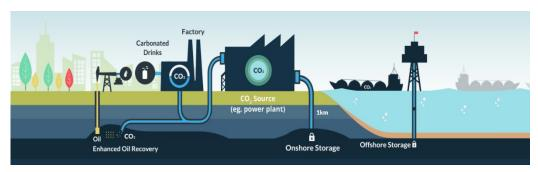
Figure 1. Scheme of the CCUS chain.
