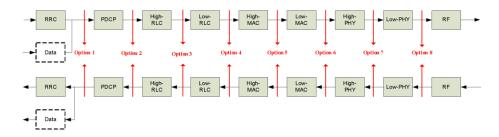
Figure 2. Function Split between central and distributed unit [8].
