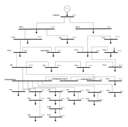
Figure 1. Electrical grid of Port of Sines
