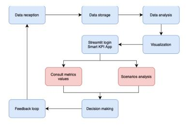
Figure 2: Data flow illustration from the data reception to the decision-making stage
