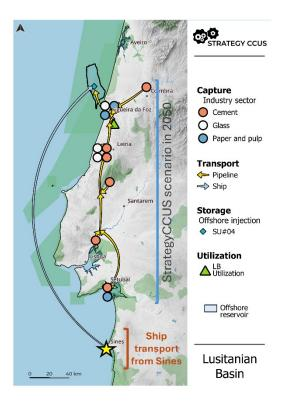
Figure 4. Strategy CCUS long term scenario with addition of the Sines cluster for ship transport.
