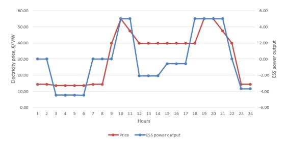
Figure 2. ESS power output.
