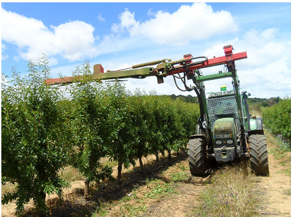
Figure 1. Summer pruning with tractor mounted disc-saw pruning machine.
