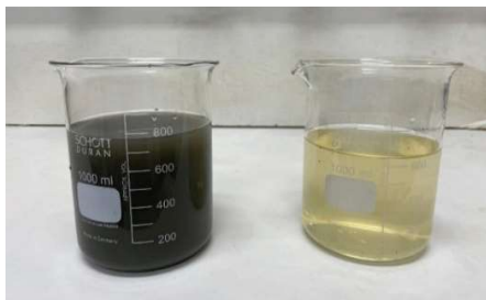
Figure 4 Mine water before (left) and after (right) Pond experiment.
