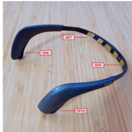
Figure 1: Electrodes position and Muse 2 headband
